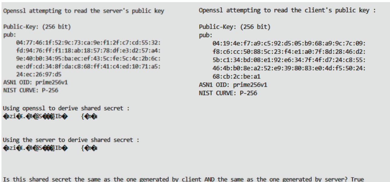
Figure 8. SERVER (top-left) & HRoT's (top-right) public key in DER format, (bottom) secret key of OpenSSL and Python SERVER
