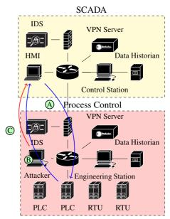
Figure 3: A generalised network diagram showing two enclaves: SCADA and Process Control.
